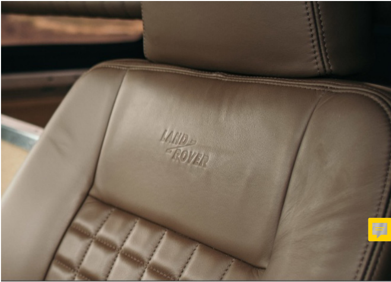
stitching & piping around edge as shown stitching no darker than leather
